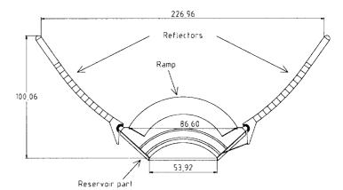
Fig. 1 Plan view of the Wave Dragon. Measures are in m.
