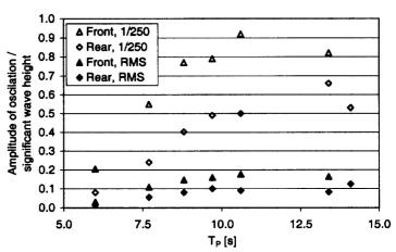
Fig. 9 Root mean square (RMS) and 1/250th amplitudes of oscillation of front and rear crest oscillations normalized by the significant wave height as a function of the wave peak period. After Martinelli & Frigaard (1999b).
