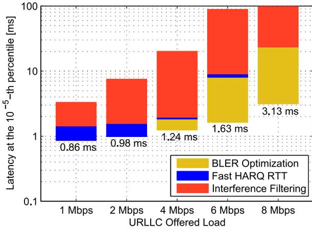
Fig. 5: Achievable latency at the  $10^{-5}$  percentile under different offered loads. The performance improvement provided by the evaluated techniques is also presented. TTI length: 0.14 ms.  $\alpha = 0.01$ .
