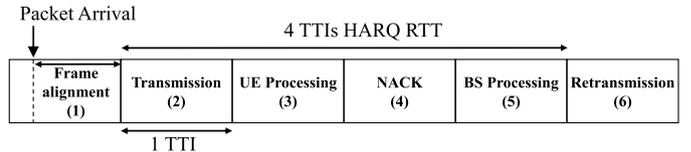
Fig. 1: Diagram of HARQ operation with 4 TTIs RTT.
