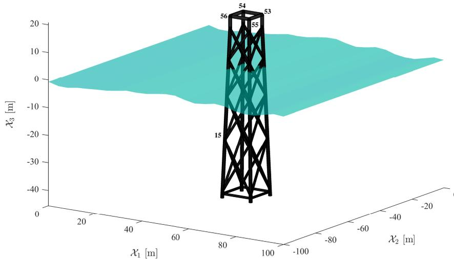
Fig. 1: FE model of bottom-founded jacket structure exposed to harmonic inputs (acting in  $X_1$ -direction) in nodes 53–56 and plane wave fields. The  $X_1$ -directional displacement response is captured in node 56. In the damaged phase, a mass perturbation is added in node 15.
