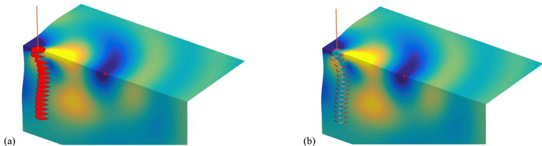
Fig. 4. Pile modelled with rigid disks (Case a) and rings (Case b), excited at 45 Hz. Soil stratification: half-space of clay. Blue/yellow shades indicate positive/negative displacements in the  $z$ -direction. The red dot is the observation point for soil displacement analysis.
