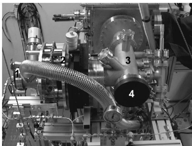
FIG. 2. Scheme and photograph of the PUCLUS: (1) pulsed valve; (2) source chamber with translator; (3) acceleration chamber; and (4) CF100 flange to place the source chamber in line with the acceleration one.
