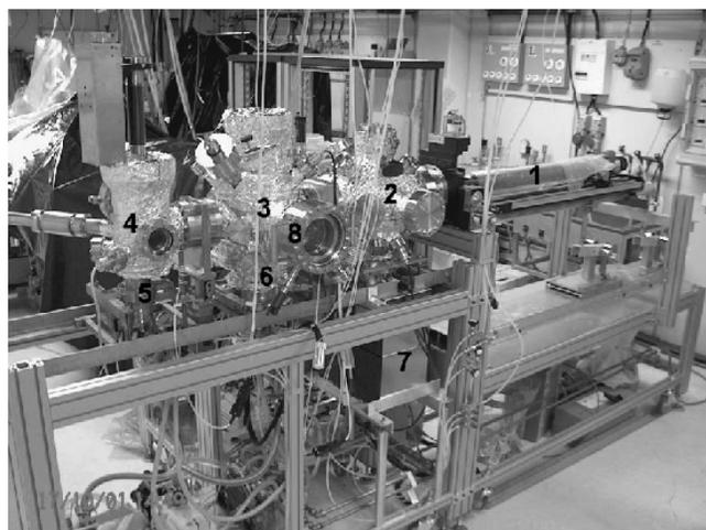
FIG. 1. Schematic diagram and photograph of the CIDA: (1) manipulator; (2) implantation chamber; (3) analysis chamber; (4) load-lock chamber; (5) and (6) turbomolecular pumps; (7) ion pump; and (8) LEED/Auger spectrometer.
