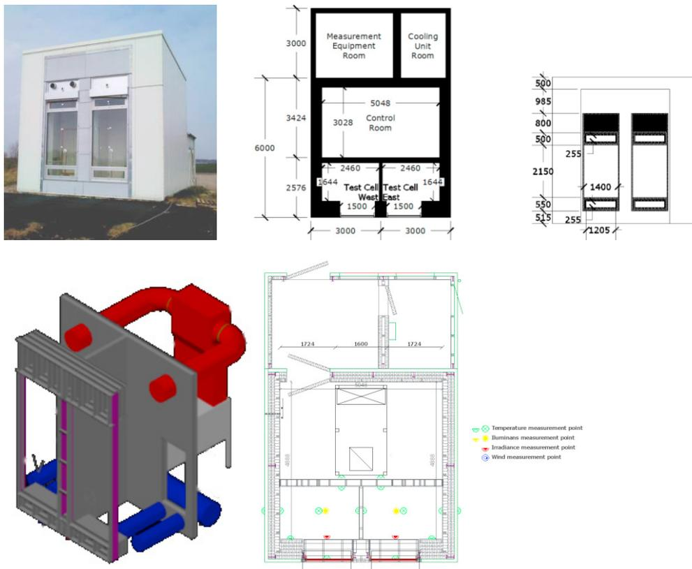
Fig. 2. Picture (left), plan drawing (center) and façade view (right) of the test facility in Aalborg.
