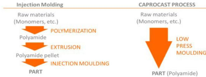
Fig. 6. CAPROCAST process compared with injection moulding process.
