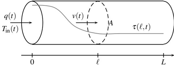
Fig. 2. Flow of heated water through a pipe section;  $\tau(\ell, t)$  is the temperature distribution in the pipe at time  $t$  and  $v(t)$  is the average speed of the water through a cross-section  $A$ .
