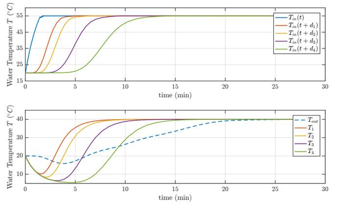
Fig. 3. Simulation with the stabilizing control law from Theorem 2. Top: forward flow leaving the supplier (blue) and reaching each consumer after delays  $d_i$ . Bottom: Outlet temperatures from each consumer. The dashed line shows  $T_{\text{out}}$ , the temperature of the return flow at the supplier
