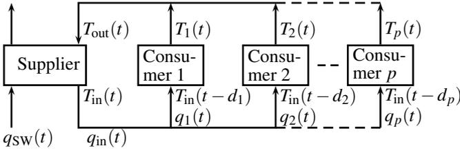
Fig. 1. District heating topology;  $q_i(t)$  are heated-water flows to the consumers at time  $t$ , indexed by  $i = 1, \dots, p$ ;  $T_{in}(t)$  is the forward flow temperature at time  $t$ ,  $T_i$  are the corresponding temperatures of water exiting the consumers' heat exchangers, and  $d_i$  are flow-dependent transport delays.
