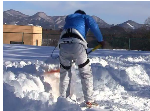
Figure 1: In the experiment, healthy participants repeated snow shoveling movement as much as possible with the aid of robot suit HAL for lumbar support. They also performed the task without HAL. Results were compared between the conditions.
