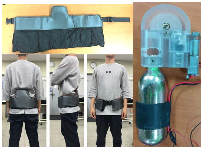
Figure 1: Air bag system and spring-trigger type inflator
