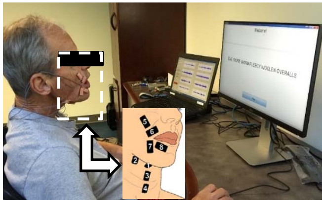
Figure 1. Subject operating data acquisition system. The callout shows the sensor location and numbering scheme.
