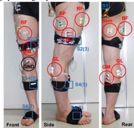
Figure 1: EMG electrode and sensor attachment locations.
