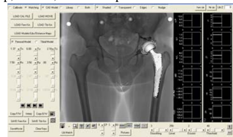
Figure 1: VA software screenshot (Kneetrack®, University of Florida, USA): cup, femur and pelvis marker-set matched on 2D contours on X-ray images for 3D pose reconstruction.
