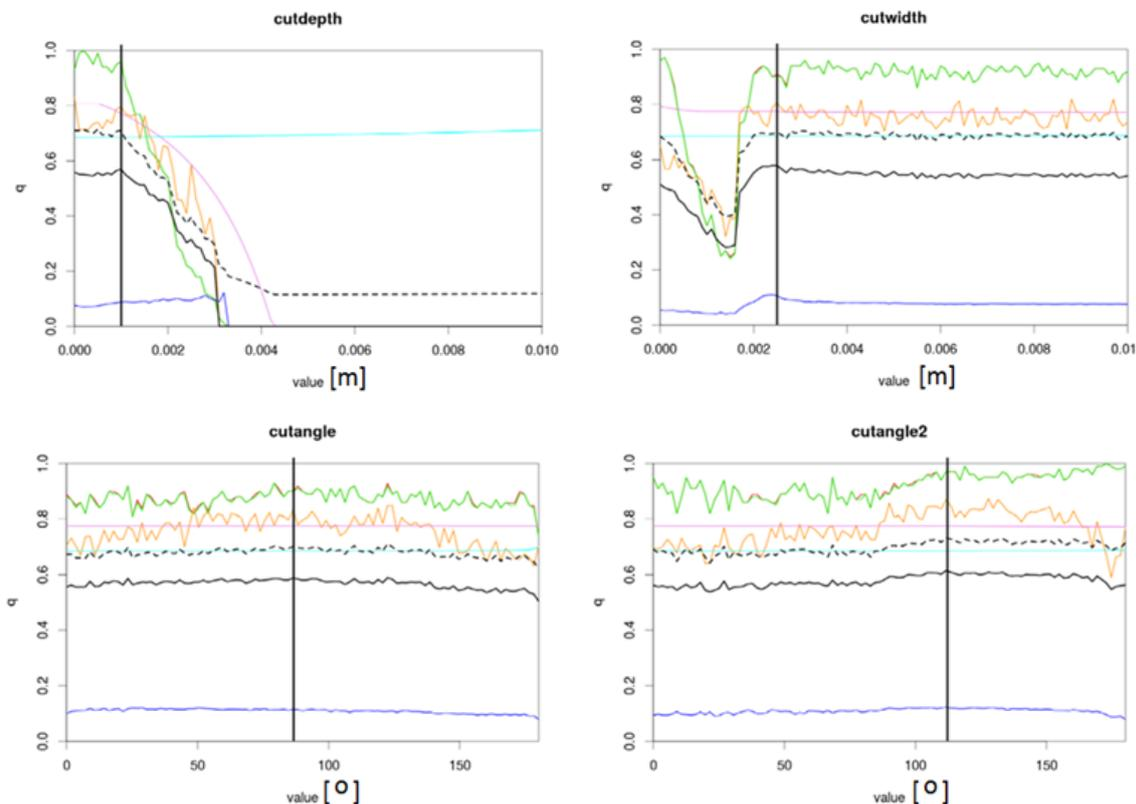
**Fig. 4.** The shape of the QI evaluations for the trapezoidal cutout parameters during the optimization process. Top row: quality evaluation for the change in cutout depth (on the left) and cutout width (on the right). Bottom row: evaluations for cutout angle #1 (on the left) and cutout angle #2 (on the right). Vertical black lines indicate the optimal values chosen for the individual parameters. Green line – Success Index, orange – Alignment Index, blue – Wrench Index, solid black –  $f(x)$
