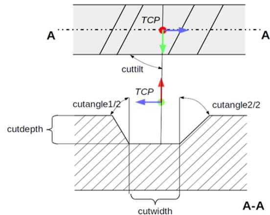
**Fig. 3.** The parametrization of the trapezoidal cutout. Top: the view of the inner surface of the finger. Bottom: the length-wise cross-section of the finger. The coordinates are defined with respect to the TCP frame shown
