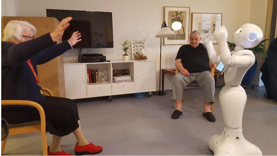
Fig. 4. Robot making an energetic expression using gestures, sound and light after successful interaction.
