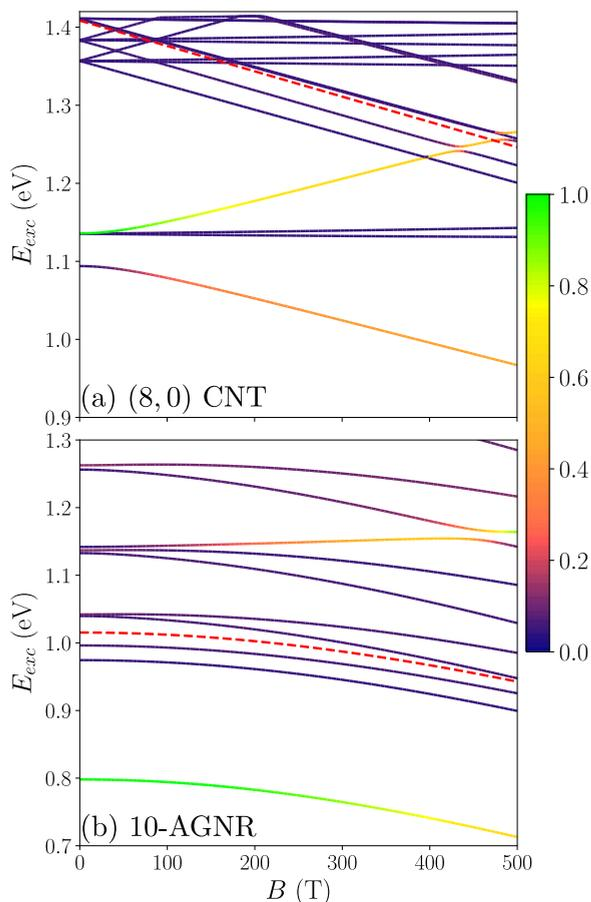
FIG. 3. Exciton energies as a function of magnetic field strength. The color of the lines in both plots corresponds to the relative optical intensity in the  $z$  direction, and the dashed red line is the band-gap energy. (a) Exciton energies of an (8,0) CNT in a parallel field. (b) Exciton energies of a 10-AGNR in a perpendicular field.
