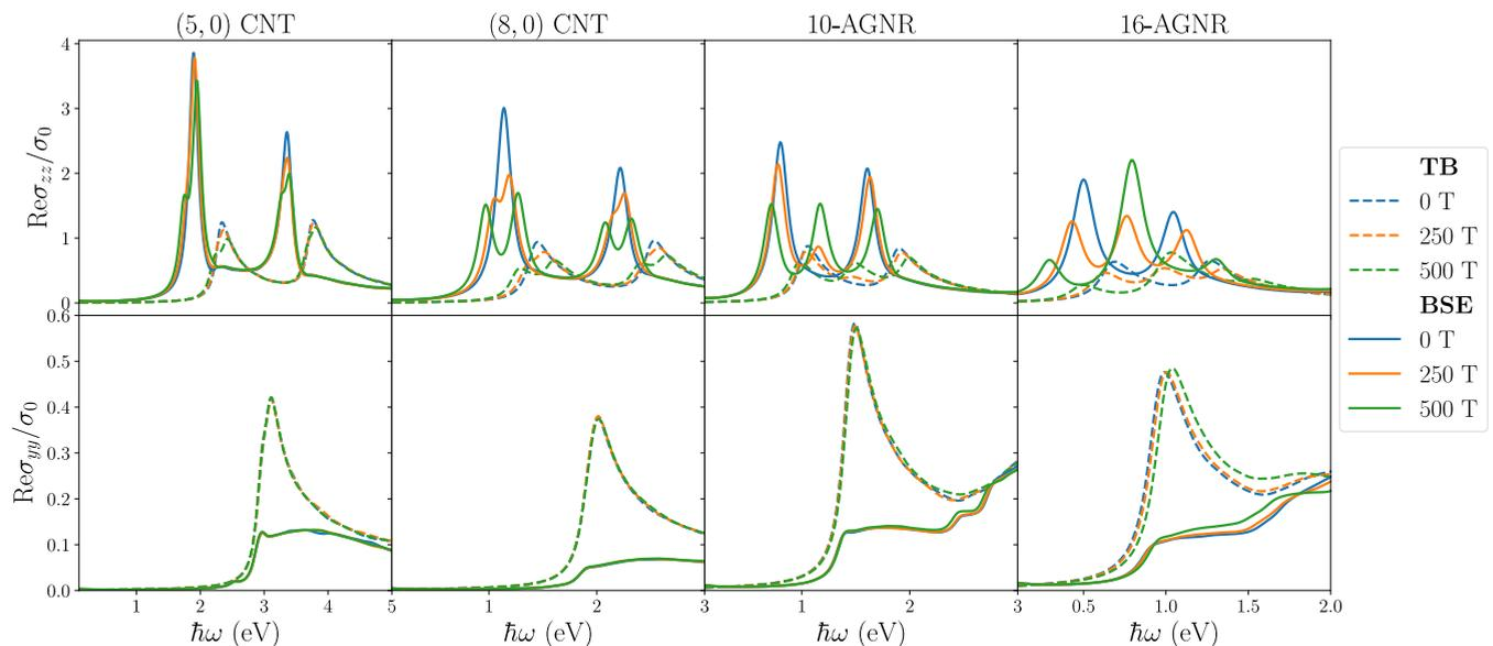
FIG. 2. Real part of the independent-particle (dashed lines) and excitonic (solid lines) diagonal conductivities  $\sigma_{zz}$  and  $\sigma_{yy}$  of (5,0) and (8,0) CNTs, and 10- and 16-AGNRs. The colors of the spectra correspond to the same magnetic field strengths in all plots. For the CNTs, the magnetic field is oriented in the parallel direction, while for GNRs it is oriented in the perpendicular direction.
