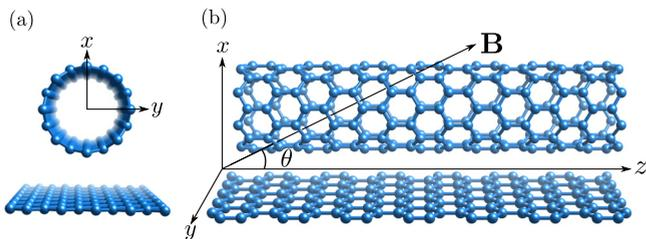
FIG. 1. (a) CNT and GNR structures as seen in the direction of the  $z$  axis. (b) Side view of the CNT and GNR structures. The GNR structure is parallel to the  $yz$  plane, with a magnetic field at an angle  $\theta$  to the  $yz$  plane and in the  $xz$  plane.
