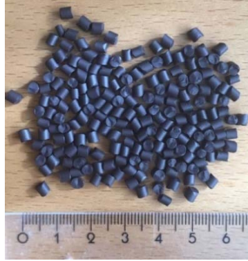
Fig.3.2_1 Raw material of ferrite magnet powder for moulding technology [8].
