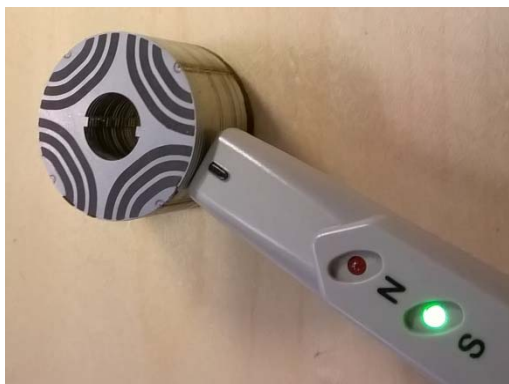
Fig.3.4.2_2 Magnetic field produced from the rotor ferrite magnet [8].
