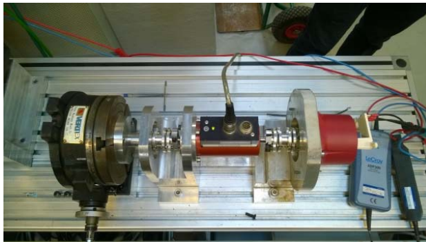
Fig.3.6.2_2 Experimental setup for torque performance measurement [8].
