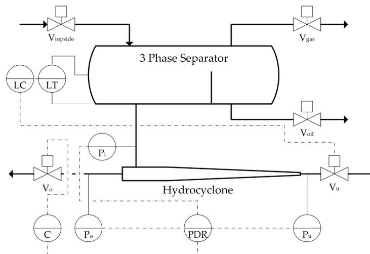
Figure 2: Two control loops in a typical control structure.
