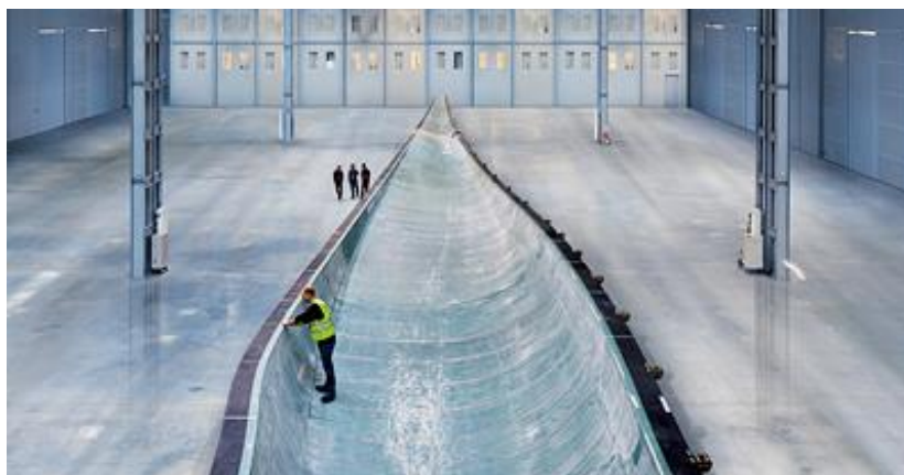
Figure 28: Mould for Siemens 75 meter blade (2012).
