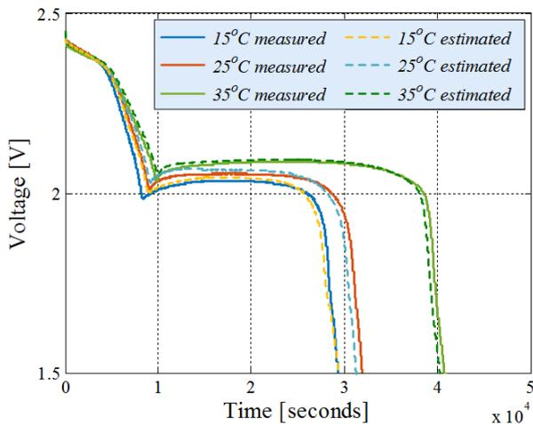
Fig. 14. Measured and estimated battery voltage for different temperatures and C/10 C-rate.
