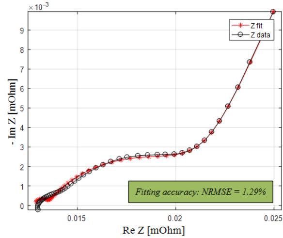
Fig. 7. Exemplification of the impedance spectrum curve fitting based on the EEC presented in Fig. 6 ( $T = 15^\circ\text{C}$  and  $\text{SOC} = 30\%$  (top),  $T = 25^\circ\text{C}$  and  $\text{SOC} = 80\%$  (middle), and  $T = 45^\circ\text{C}$  and  $\text{SOC} = 50\%$  (bottom)).
