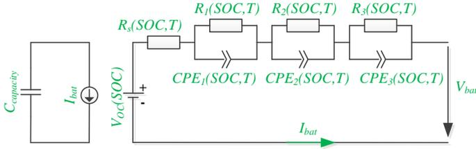
Fig. 12. ECM for estimating the Li-S battery voltage.
