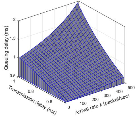
FIGURE 3. URLLC queuing delay with  $\lambda$  and  $\bar{\Lambda}_{tx}$ .
