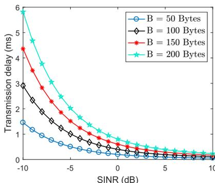
FIGURE 2. URLLC transmission delay with  $B_{llc}$ ,  $\Xi_k^{llc} = 10$  MHz.
