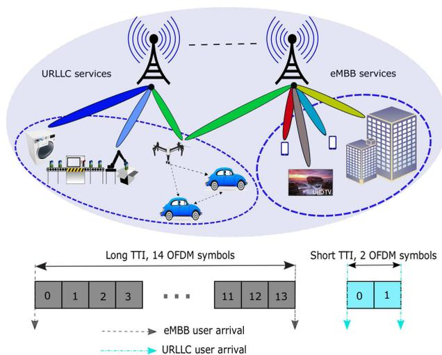
FIGURE 1. Agile 5G system model and frame structure.
