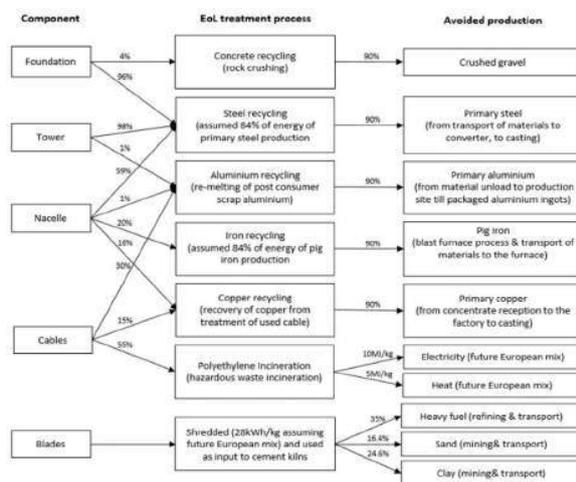
Figure 1. EoL current treatment options for wind power plant components
