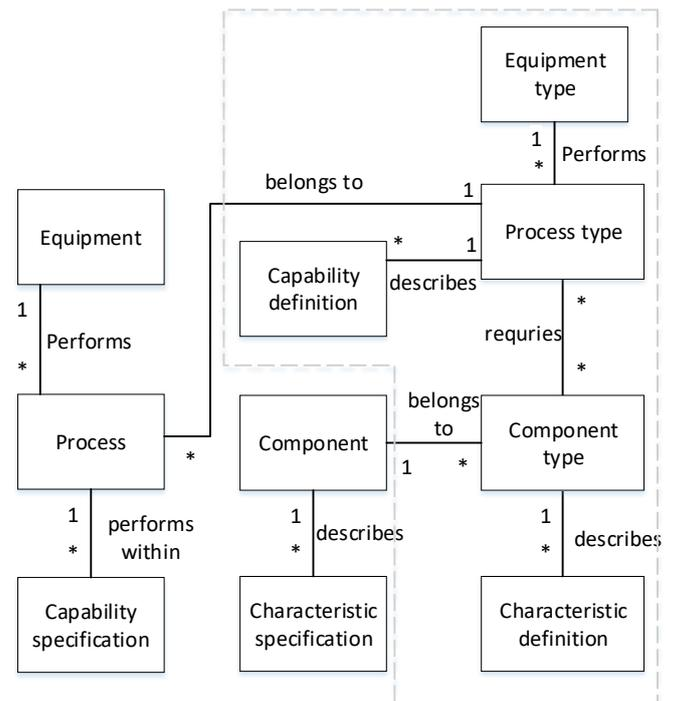
Fig. 1 UML Class diagram for product-process ontology.
