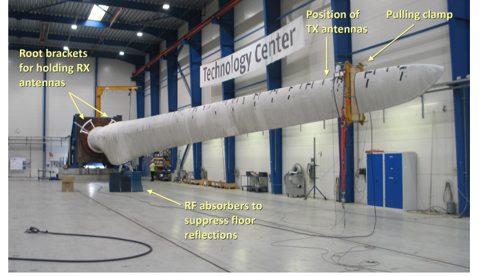
Fig. 2. Setup of Experiment 1 – the dynamic pull test. The blade can be seen from its downwind side. The cable that will be attached to the pulling clamp and perform the bending is visible lying on the floor, bottom left.
