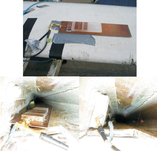
Fig. 18. Three arrangements of the TX antenna: OnGround antenna outside (top), OnGround antenna inside (bottom left) and Vivaldi antenna inside (bottom right).
