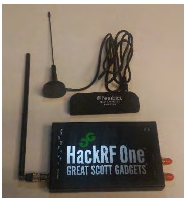
Figure 1. SDR devices: a receiver (NooElec) and a half-duplex radio.
