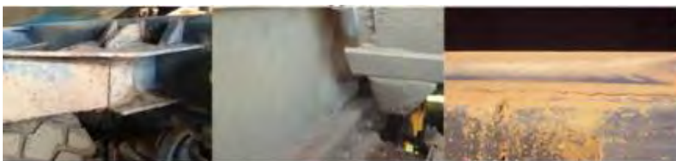
Figure 2. Crack in sub-chassis and in the bucket - Source: 69° ABM's annual congress - www.abmproceedings.com.br
