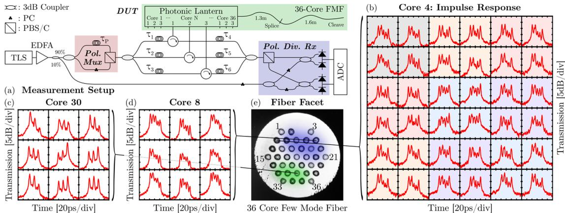
**Figure 1.** (a) Spatially-Diverse Optical Vector Network Analyzer Setup; (b)-(d) measured impulse responses: full 6×6 response of core 4, polarization combined 3×3 responses of cores 8 and 30; (e) camera image of cleaved fiber facet with core identifications and regions of different behavior highlighted.
