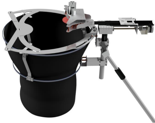
Figure 9: Portable fruit picking device designed by undergraduates in senior grades
