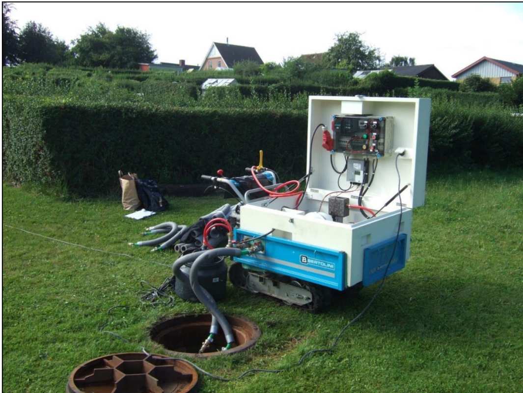
Figure 14: Ongoing TRT at the 18 m deep BHE at Langmarksvej. Inlet- and outlet pipes are insulated to prevent disturbances from ambient temperature conditions.
