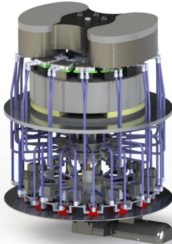
*"MagQueen" the ENOVHEAT magnetocaloric heat pump prototype*
