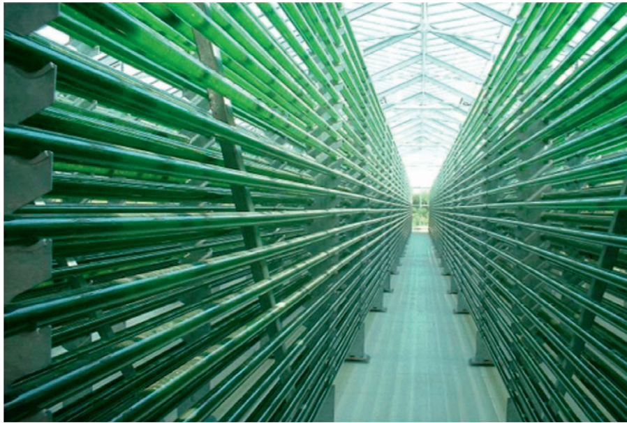
Figure 6.2 Horizontal tubular photobioreactor design (Abdel-Raouf et al. , 2012).
