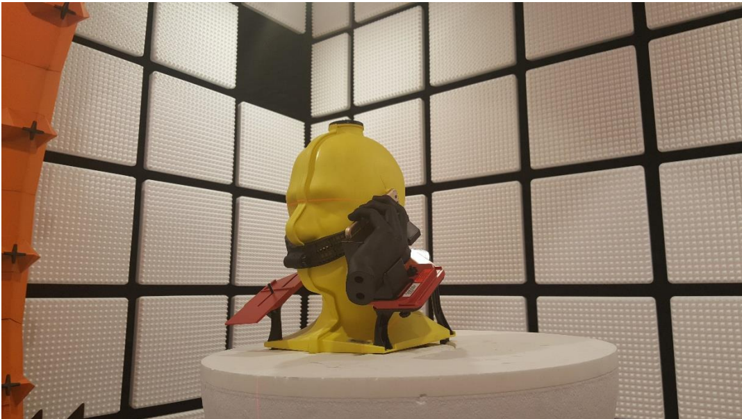
Setup for telephony with phantom head and phantom hand holding the phone.
