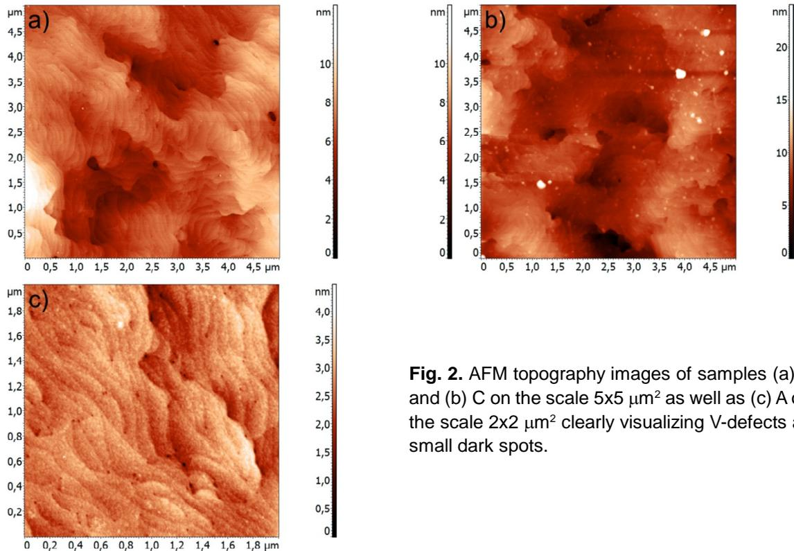
**Fig. 2.** AFM topography images of samples (a) A and (b) C on the scale  $5 \times 5 \mu\text{m}^2$  as well as (c) A on the scale  $2 \times 2 \mu\text{m}^2$  clearly visualizing V-defects as small dark spots.
