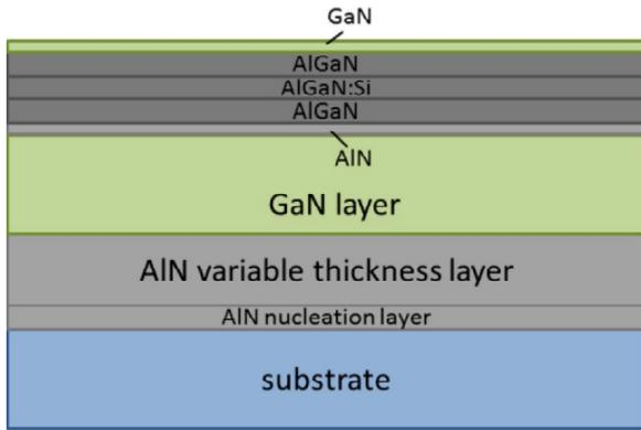
**Fig. 1.** Schematic picture of the grown HEMT structures on sapphire substrates. It includes thin (a few tens of nm) AlN nucleation layer, AlN layer of variable thickness, GaN layer of 800-950 nm in thickness, about 1 nm thick AlN capping layer, a stack of AlGaIn layers with thicknesses of a few nm each, where the middle layer is doped with Si, and about 3 nm thick GaN capping layer.
