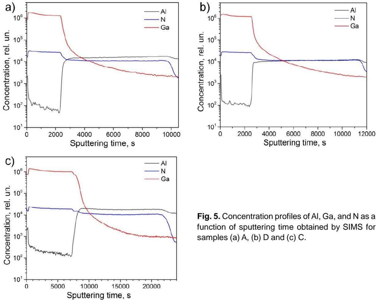
**Fig. 5.** Concentration profiles of Al, Ga, and N as a function of sputtering time obtained by SIMS for samples (a) A, (b) D and (c) C.
