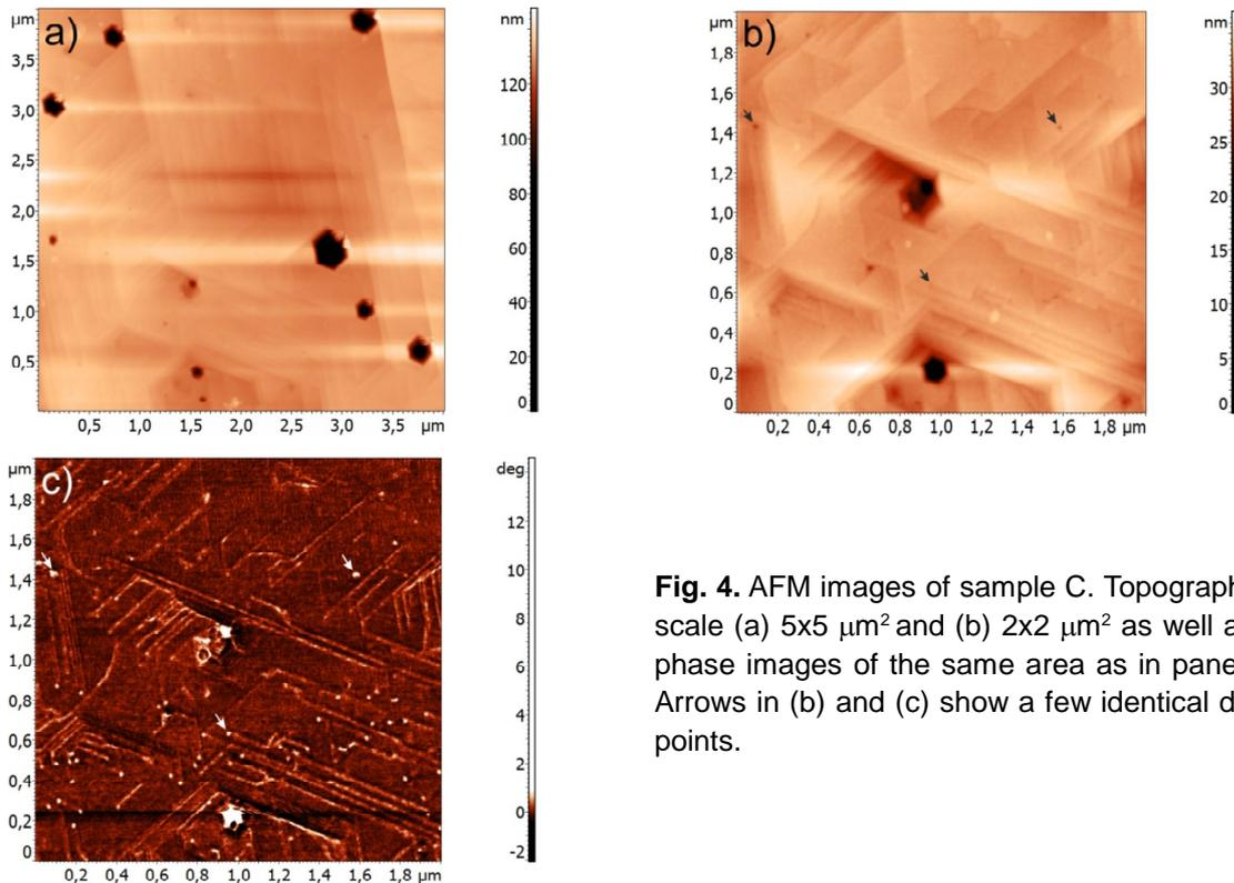
**Fig. 4.** AFM images of sample C. Topography on scale (a)  $5 \times 5 \mu\text{m}^2$  and (b)  $2 \times 2 \mu\text{m}^2$  as well as (c) phase images of the same area as in panel (b). Arrows in (b) and (c) show a few identical defect points.
