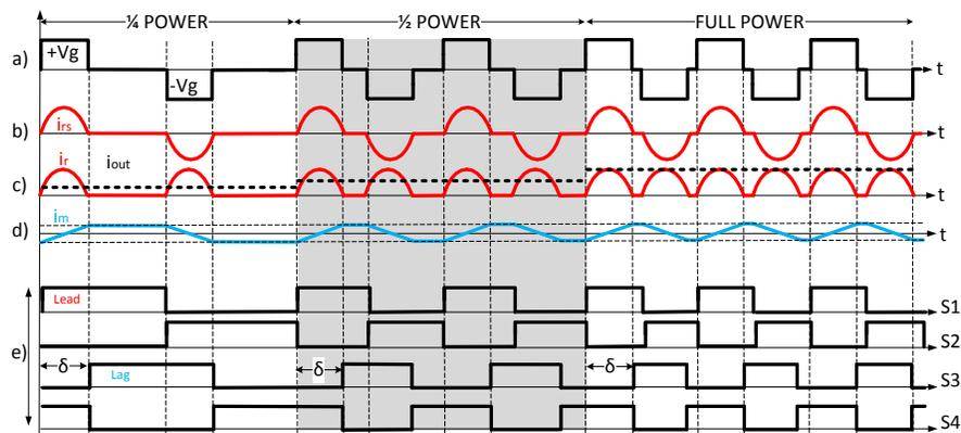
Fig. 6. Inverter output voltage  $V_g$  (a); Secondary resonant current  $i_{rs}$  (b); Rectifier output current  $i_r$  and output averaged current  $i_{out}$  (c); transformer magnetizing current  $i_m$  (d); IGBTs (S1, S2, S3 and S4) switching pattern (e).
