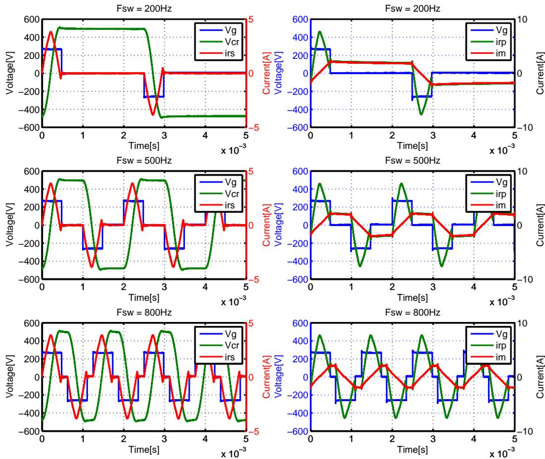
Fig. 11. Measured experimental waveforms with  $\Delta V \approx 0\%$ . Left side - measured secondary side resonant current  $i_{r,s}$ , resonant capacitor voltage  $V_{C,r}$  and inverter voltage  $V_g$ . Right side - measured inverter side resonant current  $i_{r,p}$ , magnetizing current  $i_m$  and inverter voltage  $V_g$  (b) for different switching frequencies.
