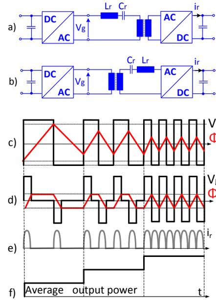
Fig. 3. SRC with tank on inverter side (a); SRC with tank on rectifier side (b); Inverter output voltage  $V_g$  and magnetizing flux  $\Phi$ , for SRC with LC tank on inverter side and frequency controlled (c); Inverter output voltage  $V_g$  and magnetizing flux  $\Phi$ , for SRC with LC tank on rectifier side and with pulse removal technique (d); Rectified current  $i_r$  (e); Averaged output power, delivered to MVDC network (f).
