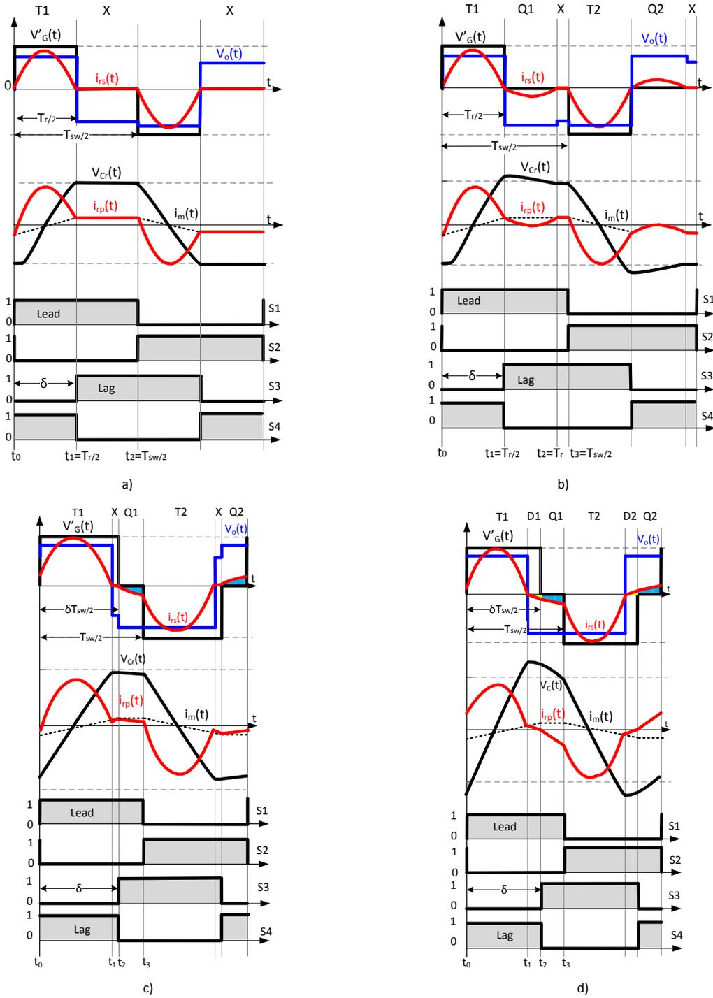
Fig. 8. DCM1 (a), DCM2 (b), CCM1-hybrid (c) and CCM1 (d) characteristic waveforms: top - inverter voltage  $V_g$ , rectifier voltage  $V_o$ , resonant secondary current  $i_{rs}$ ; middle - resonant capacitor voltage  $V_{Cr}$ , primary resonant current  $i_{rp}$ , magnetizing current  $i_m$ ; bottom - corresponding switching pattern.
