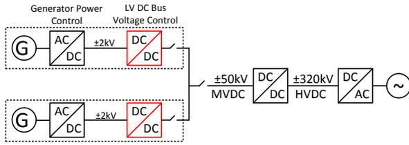
Fig. 1. Single line diagram of DC wind farm
