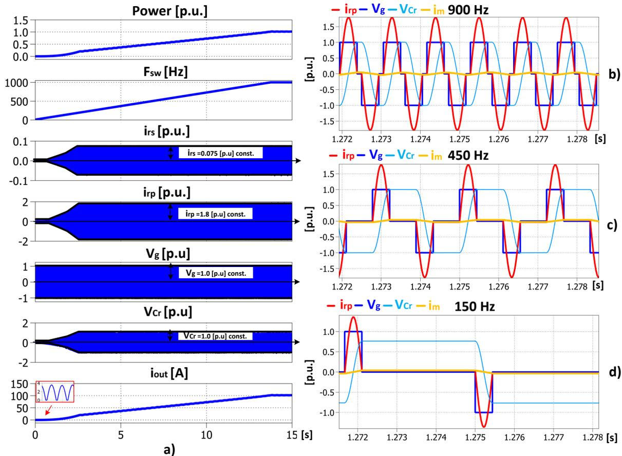
Fig. 9. Simulated results of steady state operation in DCM1 with steps in switching frequency (a); zoomed in windows of principle waveforms (primary resonant current  $i_{rp}$ , magnetizing current  $i_m$ , inverter voltage  $V_g$  and resonant capacitor voltage  $V_{Cr}$  at 900 Hz (b), 450 Hz (c) and 150 Hz (d).
