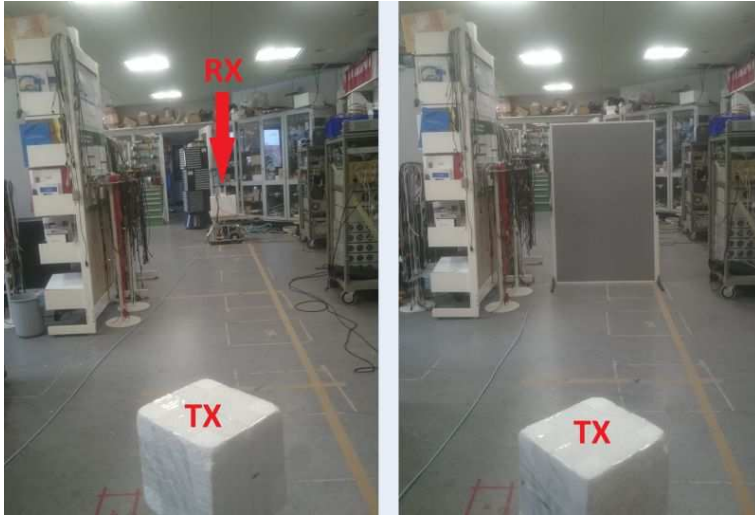
Fig. A.6: Measurement scenario. Left in the figure the LOS case is shown and right in the figure the O-LOS case is shown. The biconical TX antenna, seen in the bottom of both scenarios, is encased in styrofoam as a part of its design.
