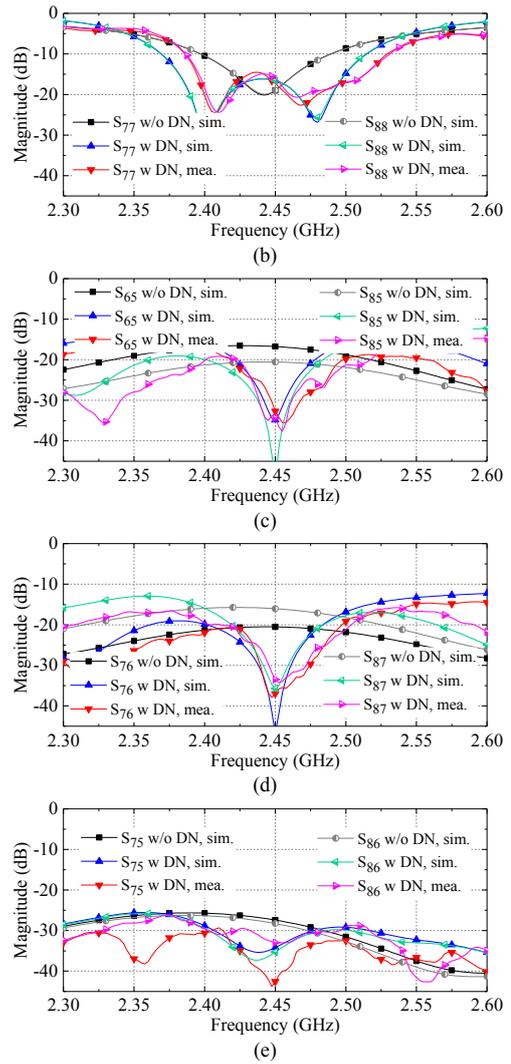
Fig. 14. Measured and simulated S-parameters of the developed prototype for the ports 5-8 with horizontal polarization. (a)  $S_{55}$  and  $S_{66}$ . (b)  $S_{77}$  and  $S_{88}$ . (c)  $S_{65}$  and  $S_{85}$ . (d)  $S_{76}$  and  $S_{87}$ . (e)  $S_{75}$  and  $S_{86}$ .
