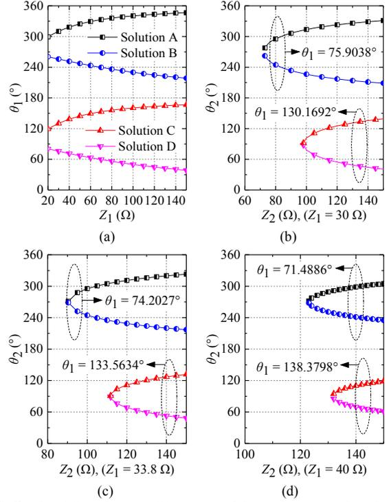
Fig. 9. Graphical formulations of the proposed decoupling network under some specified values of parameters. (a)  $\theta_1$  versus  $Z_1$ . (b)  $\theta_2$  versus  $Z_2$  when  $Z_1 = 30 \Omega$ . (c)  $\theta_2$  versus  $Z_2$  when  $Z_1 = 33.8 \Omega$ . (d)  $\theta_2$  versus  $Z_2$  when  $Z_1 = 40 \Omega$ .
