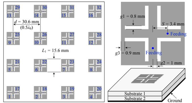
Fig. 20. Configuration of the dual-polarized  $2 \times 8$  patch array. Rogers RO4350B substrate is used for substrate 1, with the relative permittivity and thickness of 3.66 and 0.762 mm respectively, which are 2.2 and 3 mm correspondingly for substrate 2.
