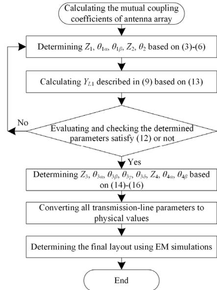
Fig. 7. Design flowchart of the proposed decoupling network for a  $2 \times 2$  single-polarized antenna array.
