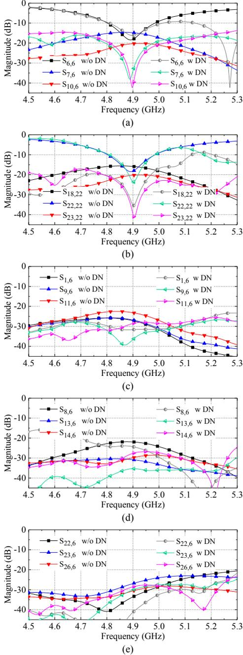
Fig. 23. Full-wave simulated S-parameters of the developed  $4 \times 4$  array. (a)  $S_{6,6}$ ,  $S_{7,6}$  and  $S_{10,6}$ . (b)  $S_{18,22}$ ,  $S_{22,22}$  and  $S_{23,22}$ . (c)  $S_{1,6}$ ,  $S_{9,6}$  and  $S_{11,6}$ . (d)  $S_{8,6}$ ,  $S_{13,6}$  and  $S_{14,6}$ . (e)  $S_{22,6}$ ,  $S_{23,6}$  and  $S_{26,6}$ .
