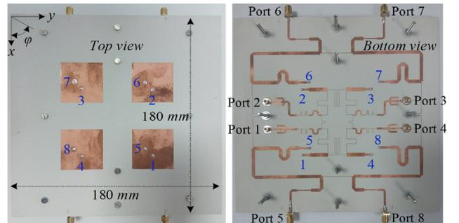
Fig. 12. Photographs of the developed 2x2 dual-polarized antenna array integrated with the proposed decoupling network.
