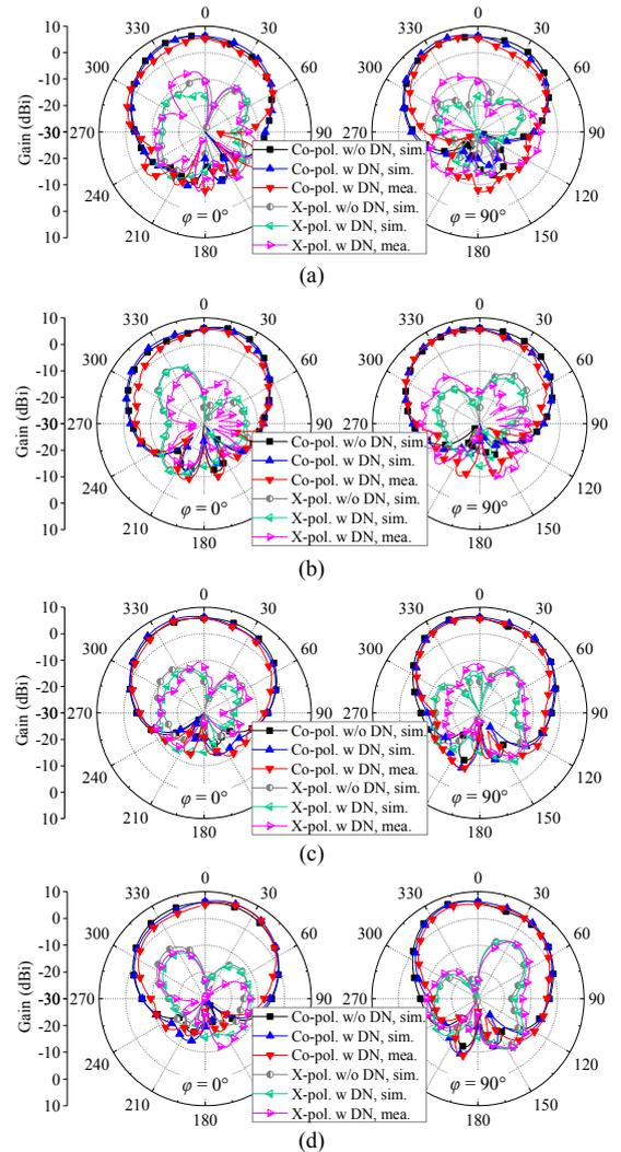
Fig. 17. Measured and simulated radiation patterns of some representative ports. (a) Port 1. (b) Port 2. (c) Port 5. (d) Port 6.
