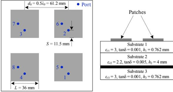
Fig. 8. Geometric structure of the employed microstrip antenna array.
