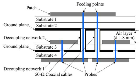
Fig. 21. Side-view of a single dual-polarized element in the  $4 \times 4$  array with decoupling network, where substrates 3 and 4 are the Rogers RO4350B substrate with the relative permittivity and thickness of 3.66 and 0.762 mm, respectively.
