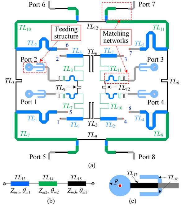
Fig. 11. (a) Layout of the proposed decoupling network for the 2x2 dual-polarized antenna array. Configurations of (b) the matching network using the classical multi-section transformer and (c) the feeding structure.
