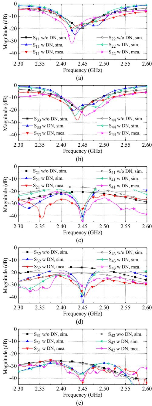
Fig. 13. Measured and simulated S-parameters of the developed prototype for the ports 1-4 with vertical polarization. (a)  $S_{11}$  and  $S_{22}$ . (b)  $S_{33}$  and  $S_{44}$ . (c)  $S_{21}$  and  $S_{41}$ . (d)  $S_{32}$  and  $S_{42}$ . (e)  $S_{31}$  and  $S_{42}$ .
