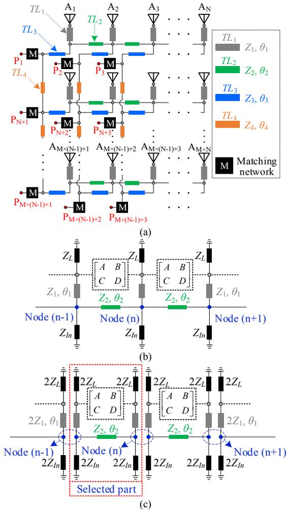
Fig. 19. (a) Block diagram of the proposed decoupling network for  $M \times N$  MIMO arrays. (b) Equivalent model between three adjacent antenna elements. (c) Simplified circuit of the model provided in Fig. 19(b) in symmetric form.
