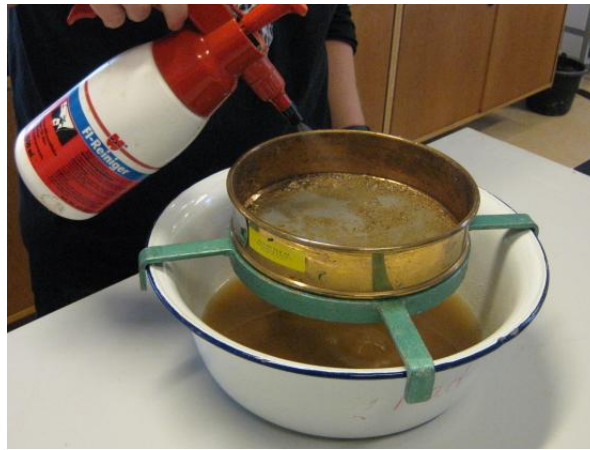
Figure 7: Spraying the silt.
