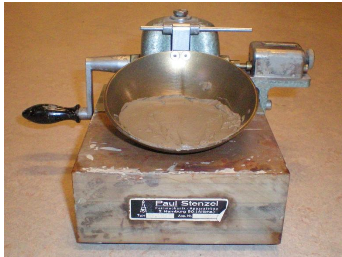
Figure 8: The sample is placed in a Casagrande Apparatus.
