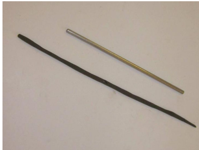
Figure 13: Roll-out and steel pin, both with a diameter of 3 mm.
