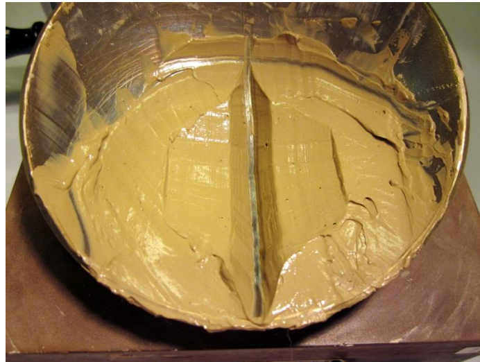
Figure 10: The groove in the sample prior to the experiment is made.
