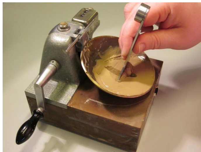
Figure 9: The groove is made over several times where the grooving tool is constantly kept right-angled on the bowl.
