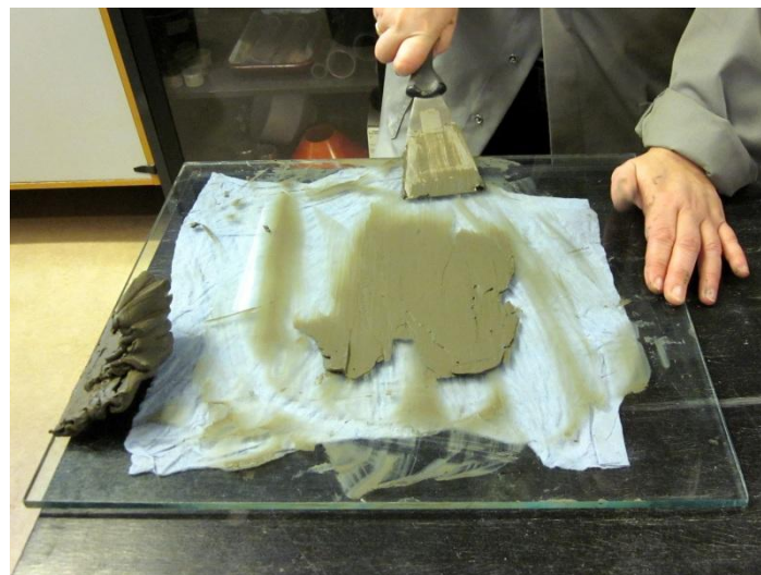
Figure 6: The sample is filled into small portions on a glass plate. If necessary, place a damp cloth under the glass plate in order to secure it.
