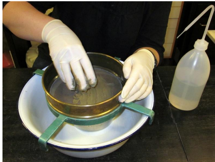
Figure 5: The sample is massaged gently through a 0.42 mm sieve.
