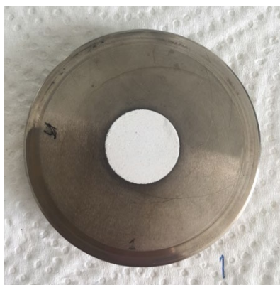
Figure 6 Tablet prepared for XRD analysis
