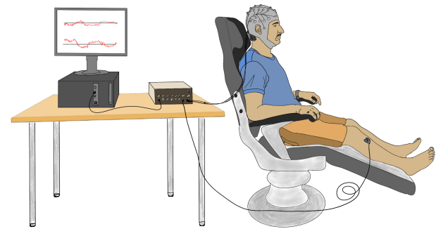
Fig. 3. An illustration of the laboratory setup for recording of EEG and sEMG data from a participant performing self-paced ballistic dorsiflexions.
