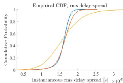
The proposed model follows the trends of the mirror source model on mean and rms delay. The constant rate model does not capture the antenna effects.
