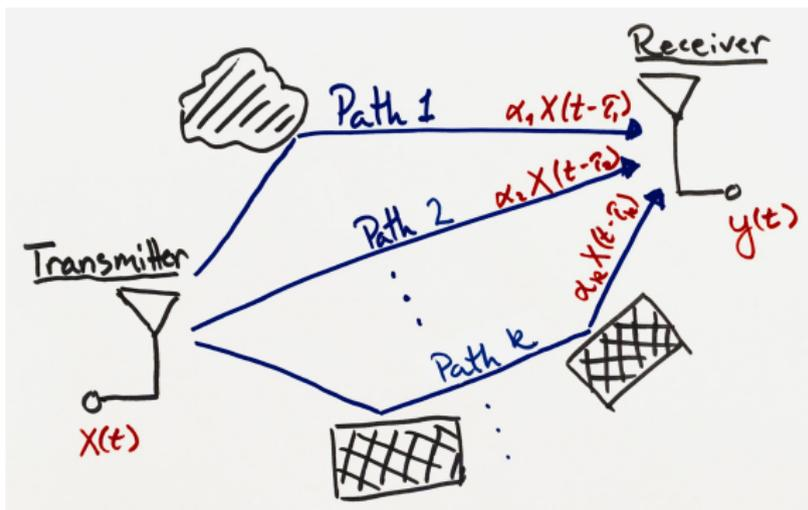
The received signal is a superposition of the multipath components
