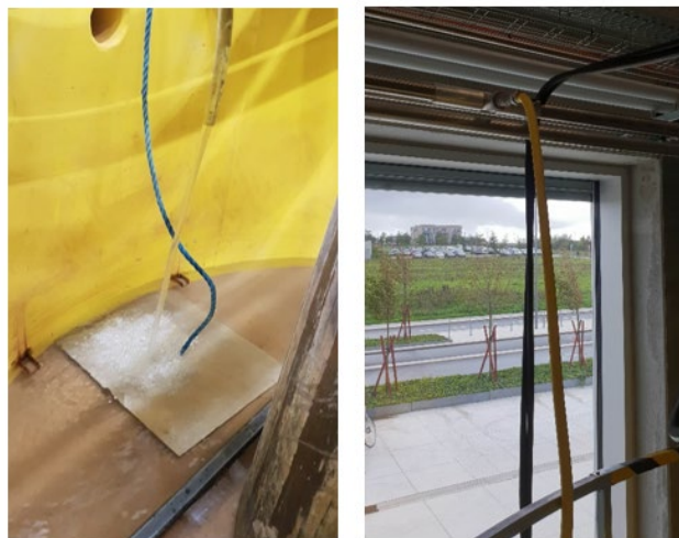
Fig. 4.7. A plate on soil surface for filling the water and water connection from the working platform
