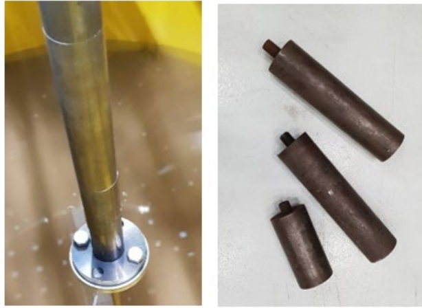
Fig. 3.5. The extension pieces for the piston
