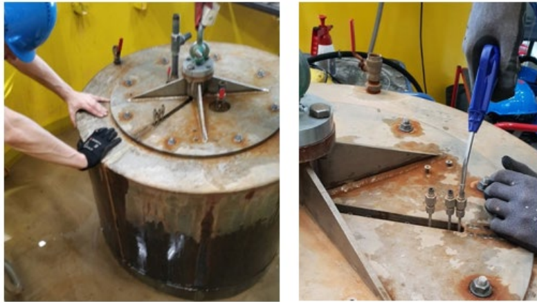
Fig. 4.11. Holding the bucket when lifting it; cleaning the bucket outlets with air piston
