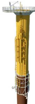
Sketch drawing of a monopile.
