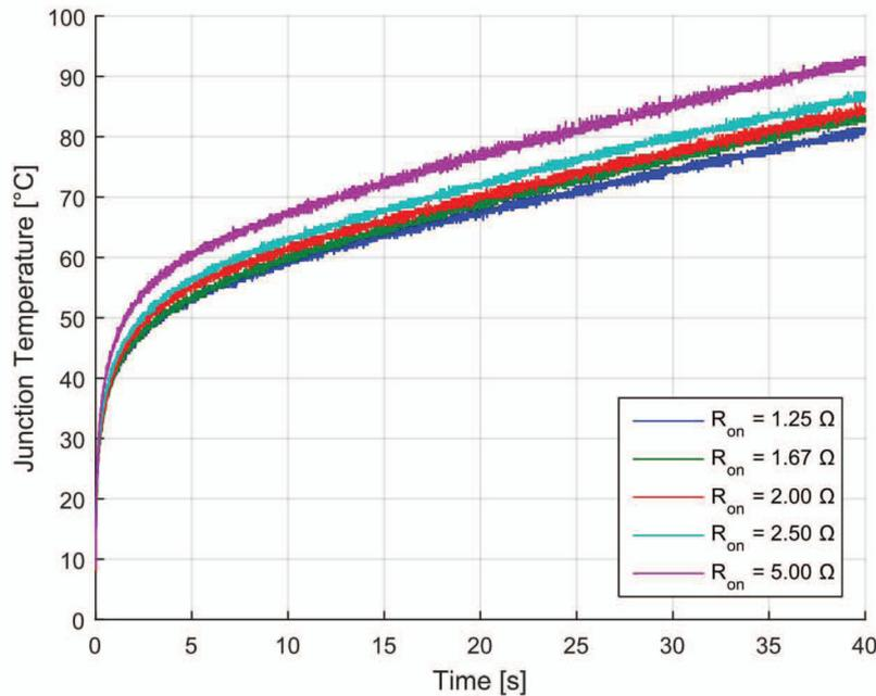
Fig. 9: Junction temperature as a function of time with various gate turn-on resistances.
