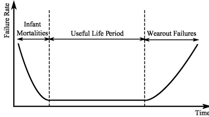
Fig. 1: Bathtub curve representing converter failure rate over time.
