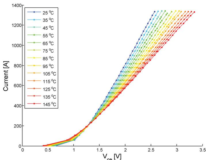
Fig. 3: IGBT I-V characteristics at different temperatures.
