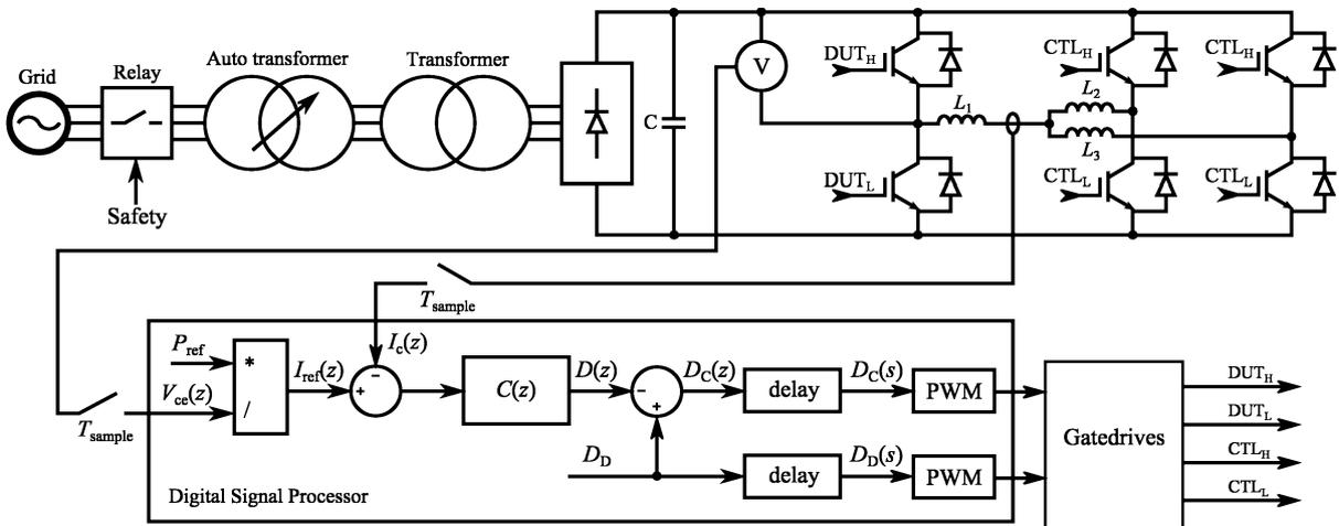
Fig. 5: Principal schematic of the test bench
