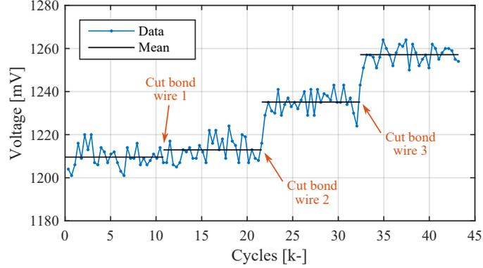
Fig. 8: On-state voltages of low side IGBT for imposed bondwire failurers.
