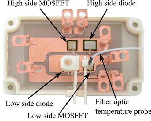
Fig. 1: Half bridge power module prototype.
