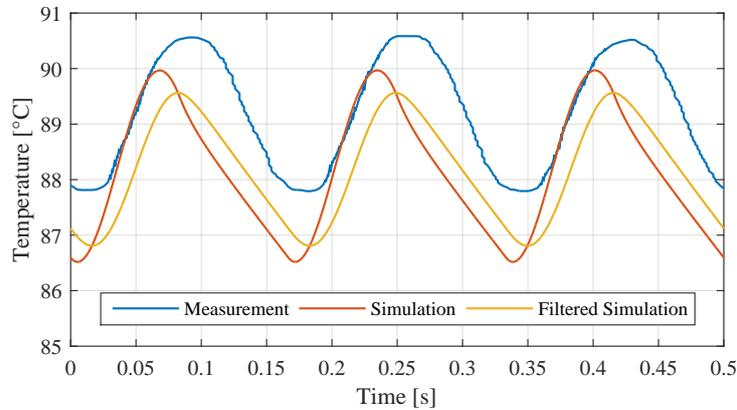
Fig. 10:  $T_s$  comparison of simulation and measurements.
