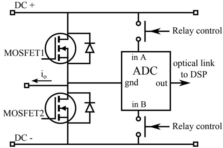
Fig. 5:  $V_{ds}$  measuring circuit proposed by [5]
