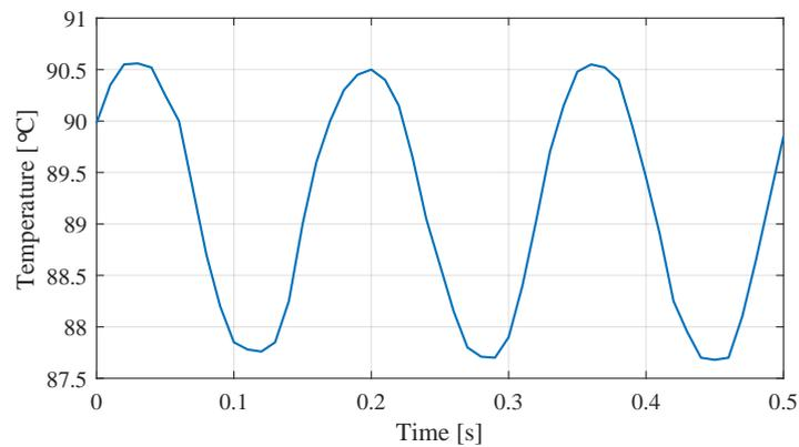
Fig. 6: Surface temperature measurement using OTG-M280
