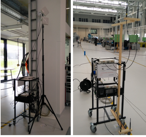
Fig. 5. Nodes of the SDR testbed. The left image shows a transmitter node and the right image a receiver node.
