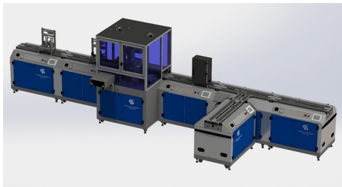
Fig. 1. Reference layout of the production line at the AAU Smart Production Lab composed of 7 interconnected modules. This number of modules translates into 14 process-specific stations as each module integrates 2 stations (one at each of the sides).
