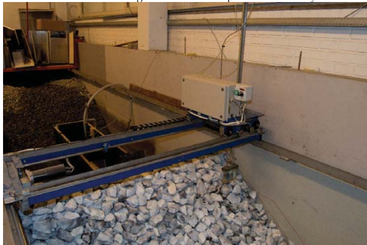
Figure 8. Profiler used to measure the eroded area.
