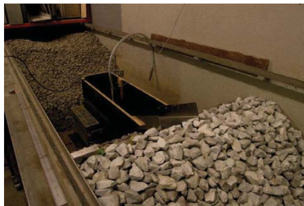
Figure 1: Set-up of overtopping tank.
