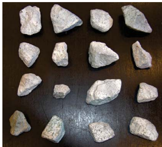
Figure 3. Class I rocks used in the armour layer for the present tests.
