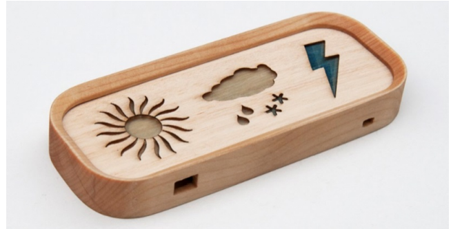
Figure 4: Electrochromic Weather Display, indicating stormy weather
