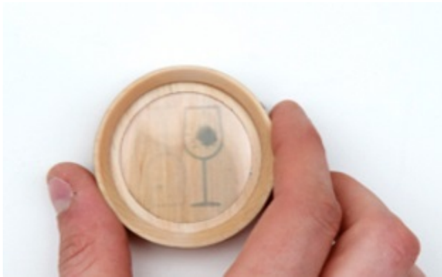
Figure 5: Electrochromic dishwasher status indicator
