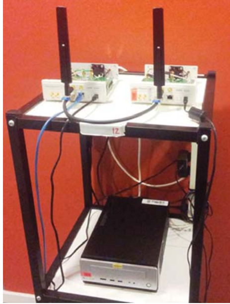
Fig. B.2: MIMO Transceiver Testbed Node.
