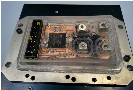
Fig. 3.27: Picture of the integrated power module after failure.
