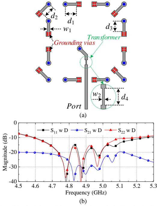
Fig. 10. (a) Physical sizes of the network layer, including the feeding line and the wavetraps, where  $d_1 = 4.5$ ,  $d_2 = 4.45$ ,  $d_3 = 4.25$ ,  $d_4 = 2.0$ ,  $w_1 = 1.0$ ,  $w_2 = 0.4$  (Units: mm). (b) Full-wave simulated S-parameters of the  $1 \times 2$  antenna array with the proposed decoupling method and the transformer for impedance matching.
