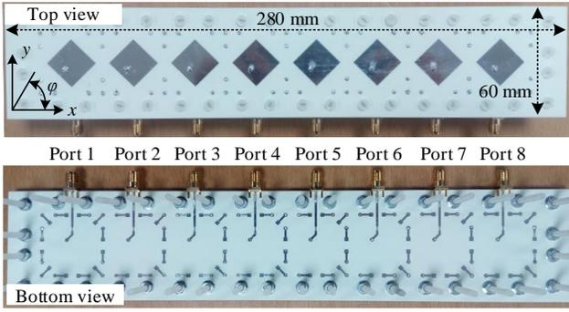
Fig. 12. Photos of the decoupled 1×8 antenna array.
