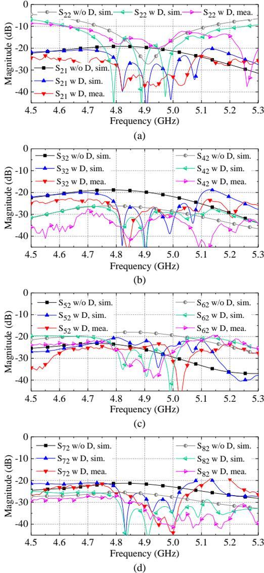
Fig. 17. Measured and simulated S-parameters of the representative ports in the 4x2 array. (a)  $S_{21}$  and  $S_{22}$ . (b)  $S_{32}$  and  $S_{42}$ . (c)  $S_{52}$  and  $S_{62}$ . (d)  $S_{72}$  and  $S_{82}$ .
