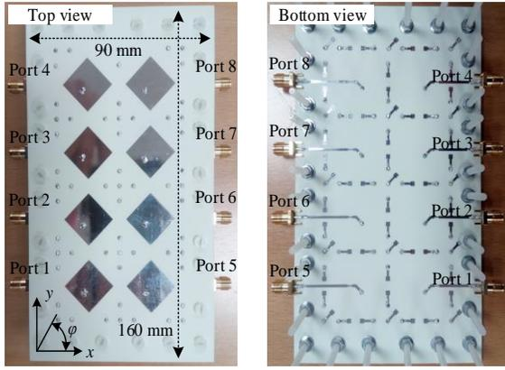
Fig. 16. Photos of the decoupled 4x2 antenna array.
