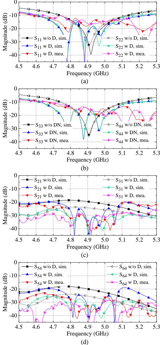
Fig. 13. Measured and simulated S-parameters of the representative ports in the 1×8 array. (a)  $S_{11}$  and  $S_{22}$ . (b)  $S_{33}$  and  $S_{44}$ . (c)  $S_{21}$  and  $S_{31}$ . (d)  $S_{54}$  and  $S_{64}$ .
