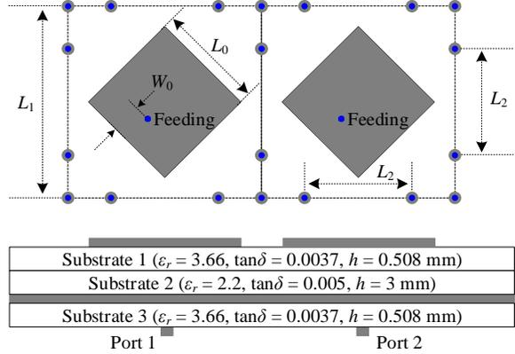
Fig. 6. Physical dimensions of a two-element patch array integrated with the proposed decoupling wavetraps, where  $L_0 = 17.0$ ,  $L_1 = 30.6$ ,  $L_2 = 17.0$ ,  $W_0 = 4.7$  (Units: mm). The diameters of the pad and the probe are 2.0 mm and 1.0 mm, respectively.
