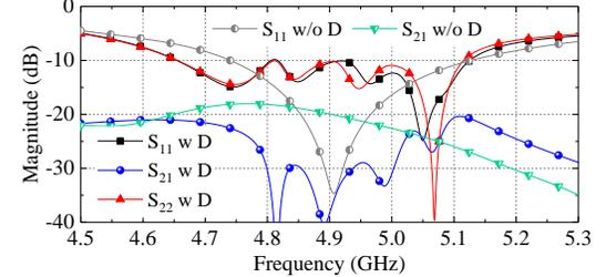
Fig. 9. Calculated transmission responses of case A with the decoupling wavetraps, where  $Z_1 = Z_2 = Z_3 = 50.0 \Omega$ ,  $\theta_1 = 50.4^\circ$ ,  $\theta_2 = 49.2^\circ$ ,  $\theta_3 = 46.9^\circ$ .
