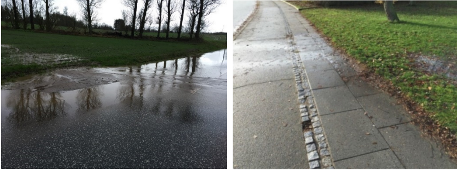
Figure 1.1. Rainfall related runoff from two pervious surfaces to impervious surfaces. Left: Runoff produced on an agricultural field flowing towards a nearby road. Right: Runoff produced from a recreational grass park in a residential area in Lystrup, Denmark.
