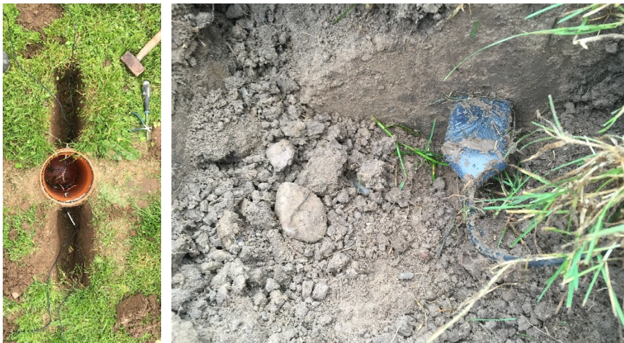
Figure 2.8. Parts of a soil sensor cluster. On the left, a vertically burried \varnothing 200 contains the data logger to collect all data from installed sensor. On the right, a mounted Decagon 5TE soil volumetric water content sensor is seen.
