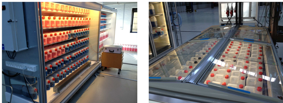
Figure 6.4: A vertical medium temperature and a horizontal low temperature display case at the Danfoss refrigeration laboratory
