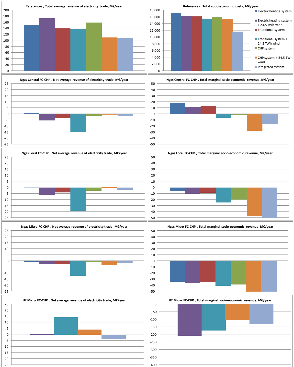
Fig. 15, Total average revenue of electricity trade and total socio-economic feasibility of the reference energy systems and net change in revenue of the four applications. Please note that the scales vary.
