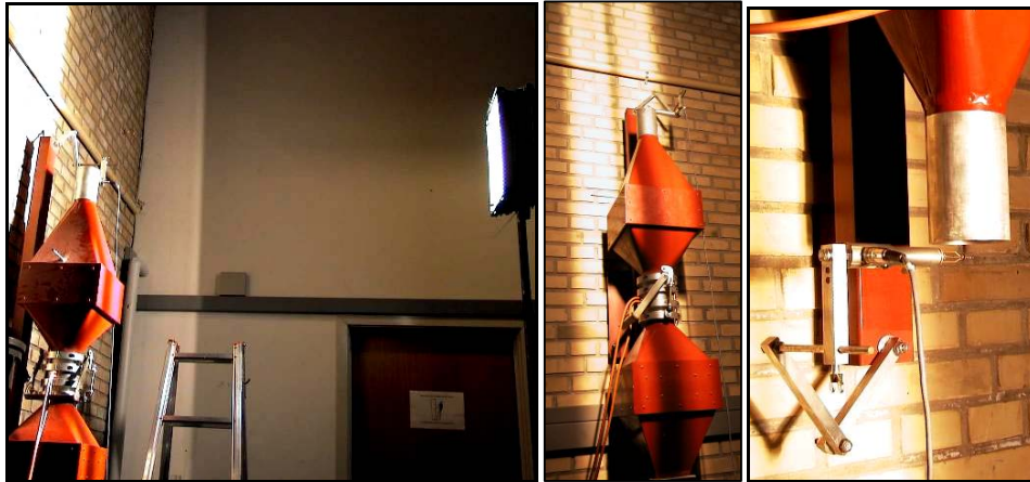
Figure 3-14. Hot-sphere anemometer in the jet-wind tunnel lit with the lamp imitating solar radiation (Jensen et al., 2007).
