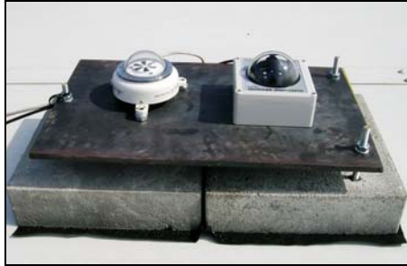
Figure 3-8. Pyranometers on the roof of 'The Cube', Wilhelm Lambrecht pyranometer at the left and BF3 at the right.
