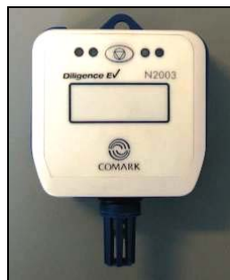
Figure 3-7. COMARK data logger N2003.
